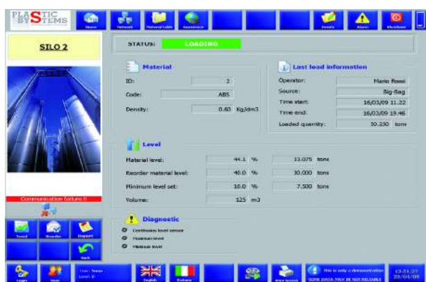
Interface for controlling silos
